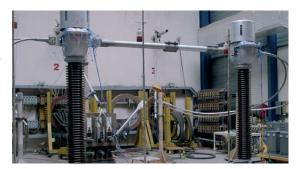
This testing facility comprises three single-phase power generators, equipped with a Varivolt transformer, whose secondary voltage on load is continuously variable. This transformer is combined with a step-down transformer delivering 50 kA current at 175 V. An intermediate output allows three-phase tests up to 5 kA at 2 kV.
