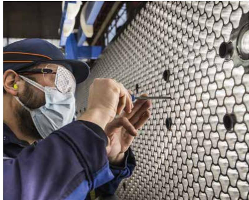
*Inspection of a steam generator spacer plate at Saint Marcel*
