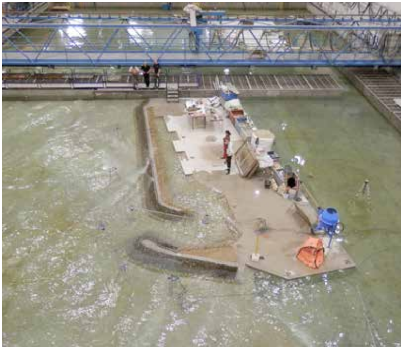
Mock-up of the Flamanville water intake channel - LNHE 34
