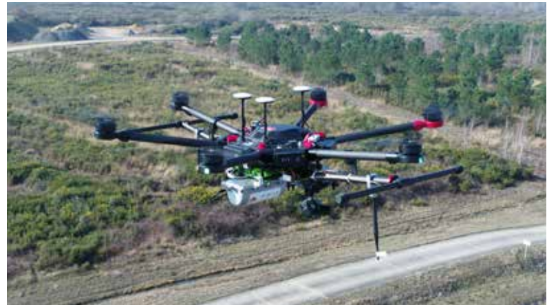
Drone equipped with a measurement probe - GIE INTRA
