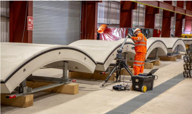
The manufacturing of the concrete segments used to line the intake and outfall tunnels is now completed. Since production began in 2019 over 45,000 segments have been produced
