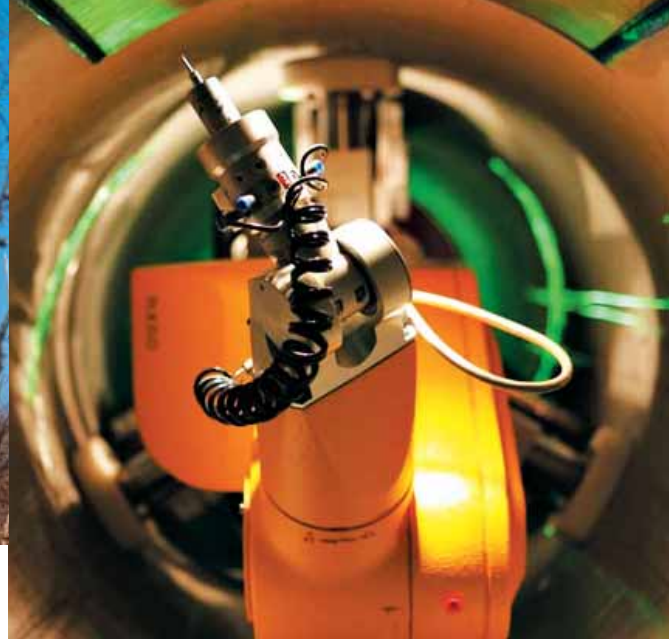
From now on, a robot will be able to reach otherwise hard-to-get-to areas of the primary circuit of the nuclear plants.
