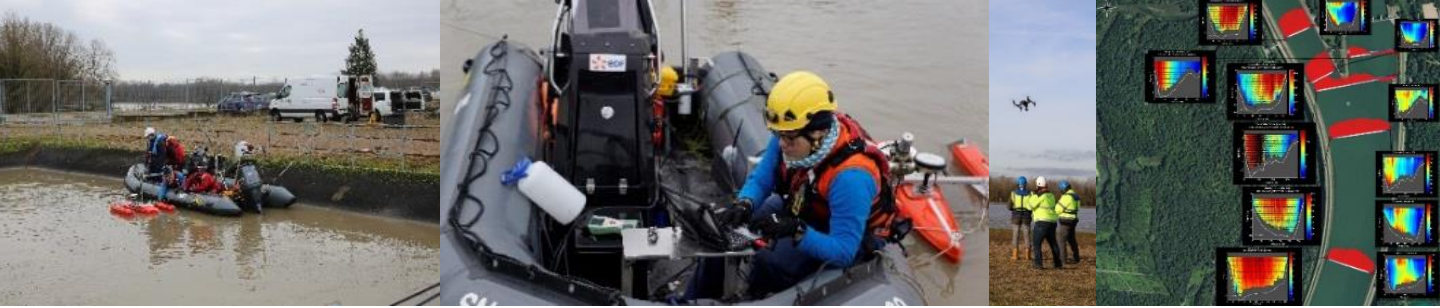
Flow characterization campaign (aDcp et in-air LSPiV) on the Rhine river, during a flood event – Rhinau dam
